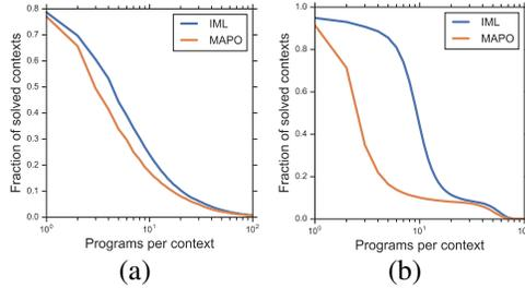
Figure 3: Fraction of total contexts for which at least  $k$  programs ( $1 \leq k \leq 100$ ) are discovered during the course of training using the IML and MAPO (*i.e.*, RER) objectives on weakly-supervised semantic parsing datasets (a) WIKITABLEQUESTIONS and (b) WIKISQL.
